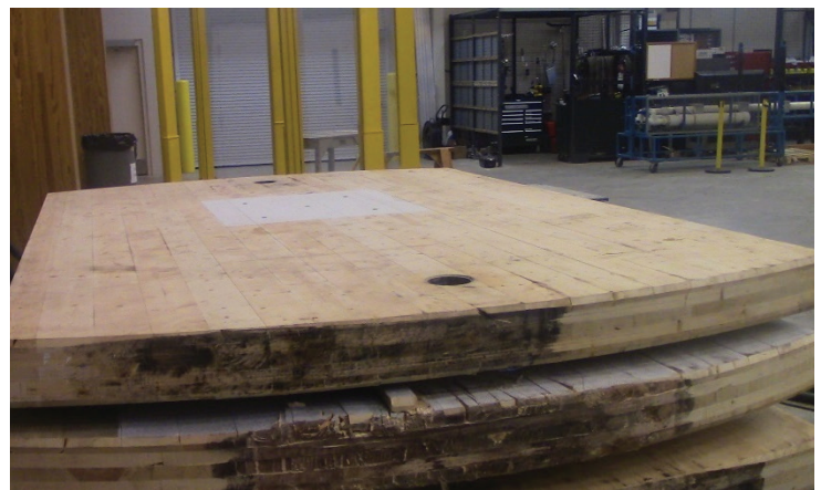
Figure 13: Bottom Edge of e = 0.73 Panel after Unidirectional Rolling Tests
