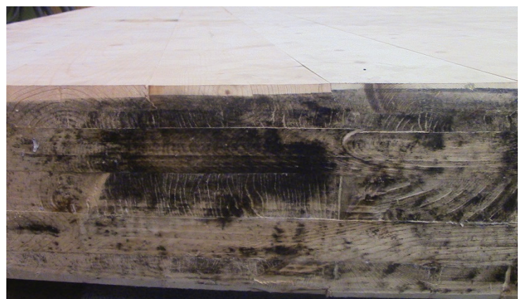
Figure 14: Local Damage of Bottom Edge of e = 0.73 Panel after Unidirectional Rolling Tests
